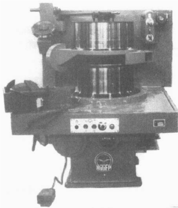
Figure 8.17 Dry wire drawing machine, Barcro system, driven by the worm gear drive designed and manufactured by DIGÉP
